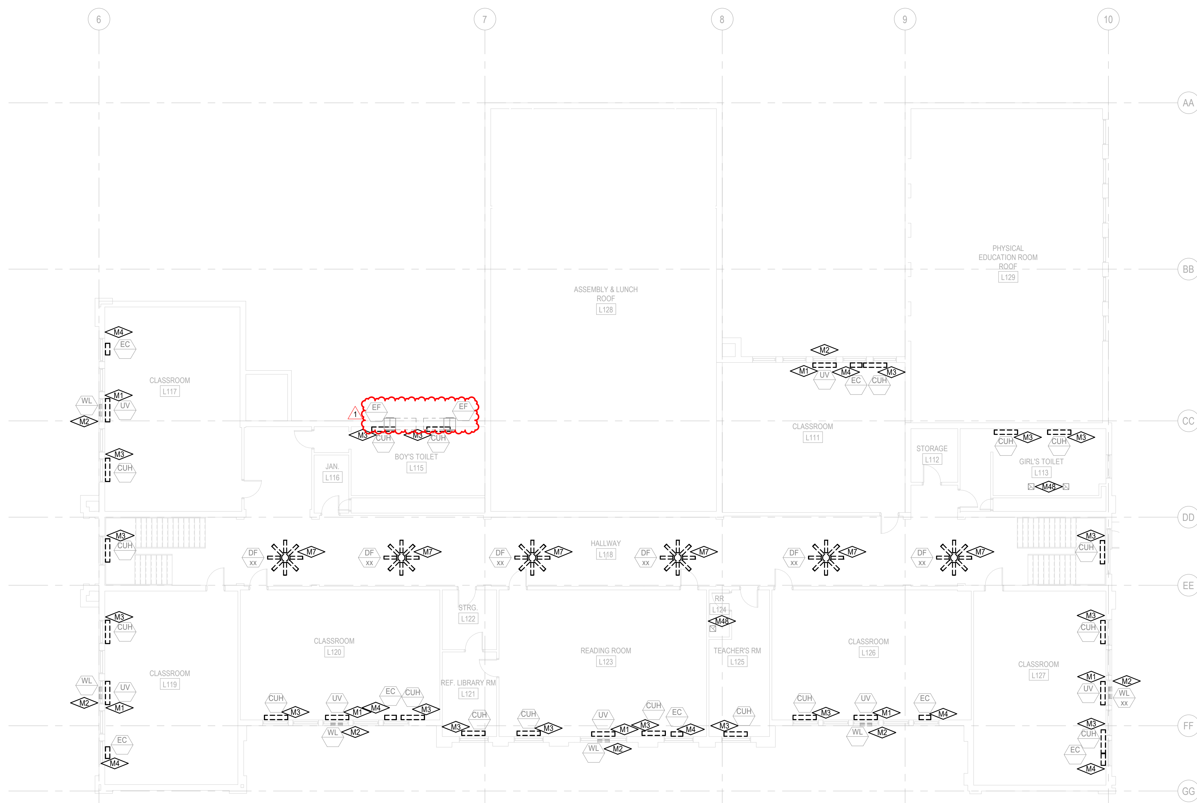
LEVEL 02 - COMPOSITE HVAC DEMOLITION PLAN SCALE: 1" = 10'-0"
